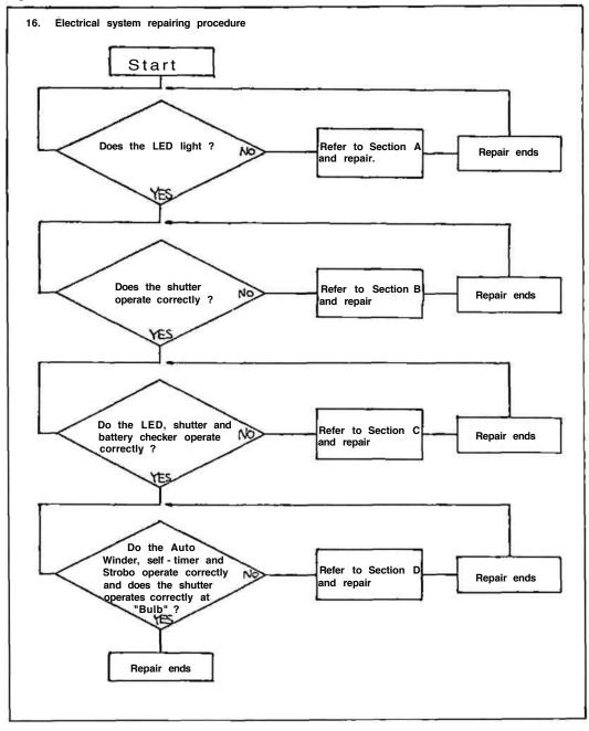
16. Electrical system repairing procedure Fig. 78
