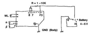
After winding up the film advance lever, apply voltage to terminals of the M printed board as shown above, and see if the moving contact is held firmly or not. When the moving contact is held firmly, the condition is normal.
