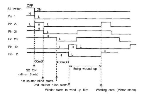
NOTE: During winding up operation, (L) signal is sent to pin 2 from the auto-winder and when (L) signal is on pin 2, the mirror starting is prohibited. As soon *as* the winding is completed, signal is switched over to (H), causing the mirror and shutter to start.
