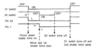
NOTE: With the Tr2 and Tr3 circuit, the mirror and 1st shutter blind start when the S2 switch turns on. The 2nd shutter blind does not start even if the S2 switch turns off, but it starts when the SI switch turns off also.
