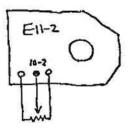
With the F - potentiometer connected to the camera body, make sure that 2.5V is delivered to pin 5 of the HA16517, and check the battery for voltage. Next, turn the focusing ring and make surethat voltage on terminal 10-2 of the E11 - 2 switch varies about 1.0 to 1.8V. (80 mV/EV; Voltage is lower at F1.4 side)
