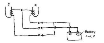
Apply voltage to the lead wires pt the  $\mathbf{1}$  and  $\mathbf{\beta}$  magnets as shown above, and see if the moving contacts are held firmly. When the moving contacts are held firmly, the condition is normal.
